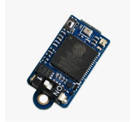
Nano V1 Tiny altimeter photo found on Model Rockets ( https://modelrockets.co.uk )
